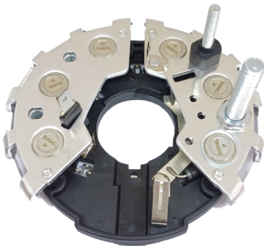
FA-B-0928 Placa Bosch 1127320664 /-665 /666 /-695 /-926 VW, Case, Termo King. CON DIODO AUXILIAR
