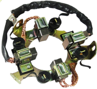
PCB-01 S/Carb. PCB-01-1 C/Carb. Camion Ford Arr. MWM Cod 246.007 EX-213-13 Fijacion:
